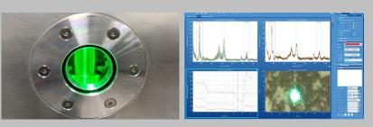
Vacuum chamber with in-line Raman and profiler Raman spectrometer data on a wear mark.
