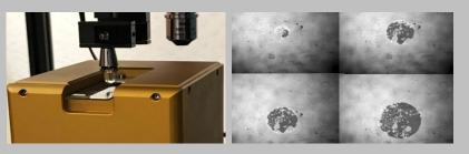
A test showing hydrogel against a coated glass slide. Real time contact area analysis vs force.
